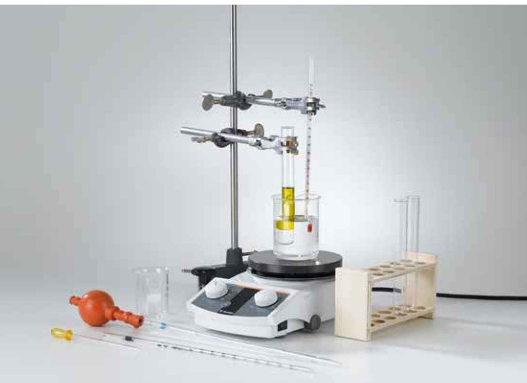
Production of fuel from rapeseed oil (C5.4.1.1)
